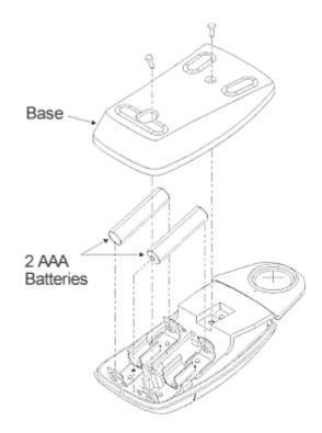
**Note:** When you replace the cursor batteries, the cursor will reset to the default frequency. If you changed the frequency of the cursor before replacing the batteries, you will need to do so again after replacing the batteries (see the Reducing Monitor Interference section in Solving Problems).
