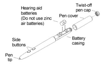
**Note:** When you replace the pen batteries, the pen will reset to the default frequency. If you changed the frequency of the pen before replacing the batteries, you will need to do so again after replacing the batteries (see the Reducing Monitor Interference section in Solving Problems).
